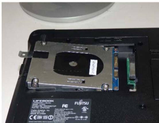
LH531 Removing Old Drive
